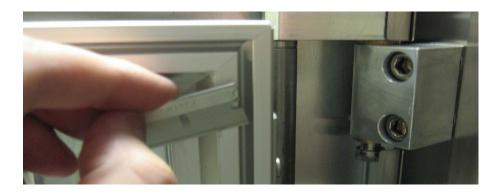
Step 3 – Clean up the door frame. Any excess silicone can carefully be removed using a razor blade. Wipe down the frame to help clean up excess dirt debris.
