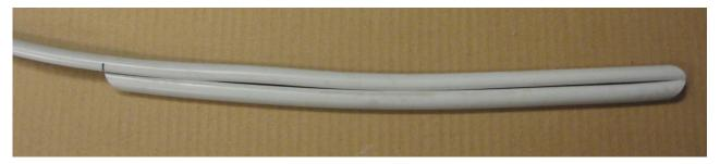
Step 5 – Measure 5/8" of an inch from the end of each piece of gasket and make a line marking with black marker. Using a blade cut the gasket at a 45 degree angle using the line marked as a guide. It is important to note that when cutting the gasket angels that you make the same inward facing cut on both ends. As shown above. The bottom gasket has both angels facing inwards.
