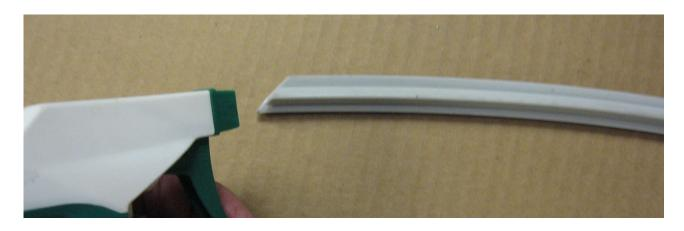
**Step 6** - Install the door gasket by lubricating either the dart or T piece of the gasket with a mixture of soap and water. This will allow you to be able to install the gasket much easier and quicker. If you notice any portion of the gasket does not seem to pop in you can take a cylinder and roll it along the gasket to help fit the gasket into the frame.
