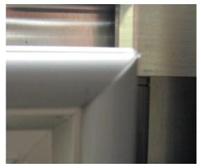
**Step 7** – Line each corner up as evenly as possible. The gasket should be wiped clean at this time and make sure before proceeding to the next step the gasket comes to a complete dry.
