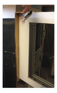
Step 1 – Open the oven door. Place a piece of cardboard or non-abrasive material between the oven door and the face of the oven to help prevent the door from damaging the face of the oven.
